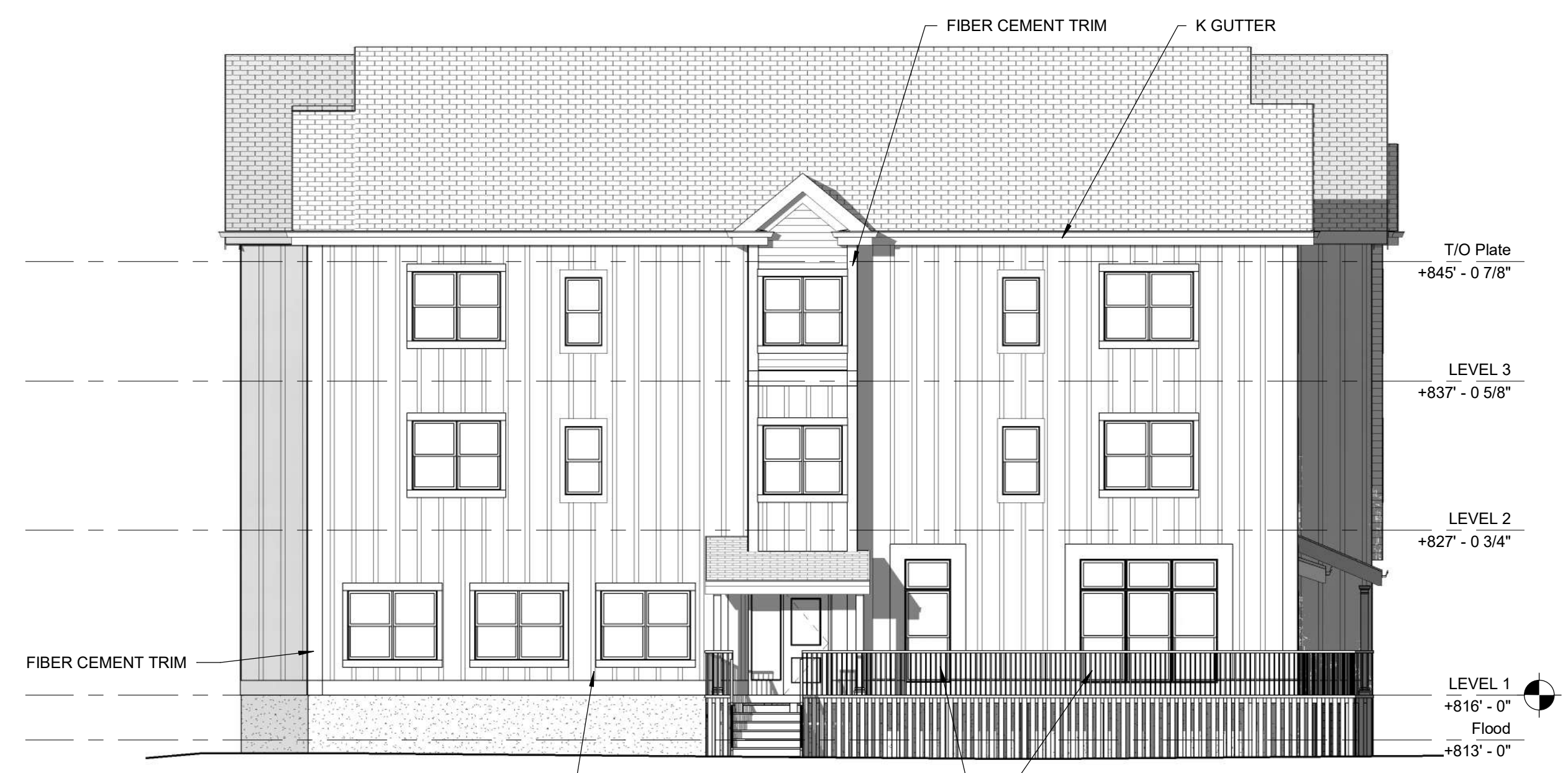
2 EXTERIOR ELEVATION - NORTH 1/8" = 1'-0"
